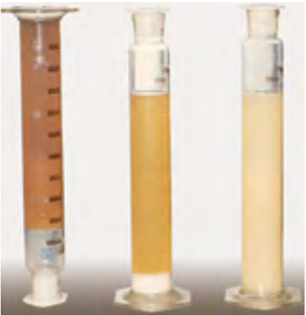
a) = Diesel without antifreeze (Solid not pumpable) b) = Diesel with traditional antifreeze (observe sedimented paraffins) c) = Diesel with Arctic (no sedimentation of paraffins)
