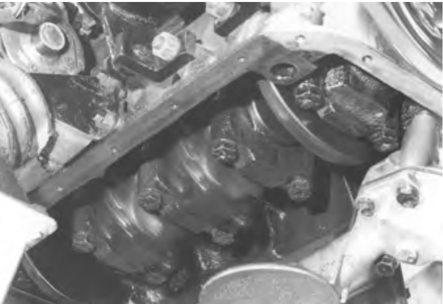
A picture of one of the many tests conducted on engines without hydrodynamic lubrication (without oil) and previously treated with Sintoflon. Observe the connecting rods.
