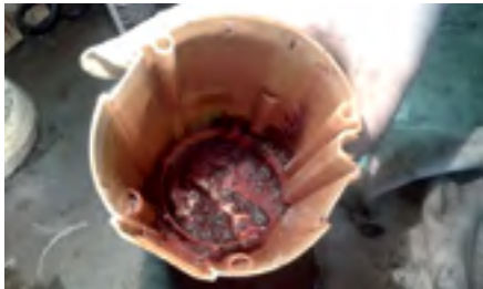
Photo of contaminated Diesel pump . The problem becomes even worse in case of sporadic use of vehicle.
