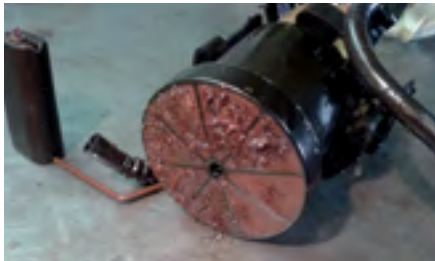
Photo of contaminated Diesel pump . The problem becomes even worse in case of sporadic use of vehicle.
