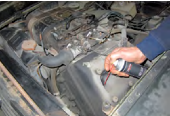
Drylube when sprayed into the cylinders through the spark plug hole is ideal for lubricating and unlocking pistons, piston rings etc. Ideal for engines after long periods of stop for instance on historic vehicles.
